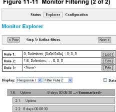
**Note:** Some devices might use a variable number of lines to display status depending on the device state. If so, slicing first by lines will not consistently point to the desired data. Instead, consider a different strategy:
